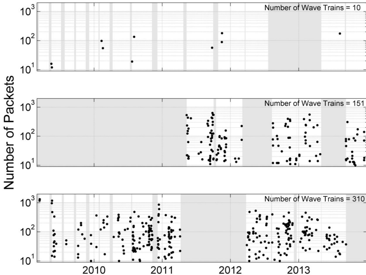
Figure 4. Number of MFAS packets (black dots) in each wave train over the five year study period for site M (top), site H (middle), and site N (bottom). Light gray regions are periods that were not analyzed (see Table 1). Note the vertical axes are logarithmic base-10 from 10 to 2,000.
