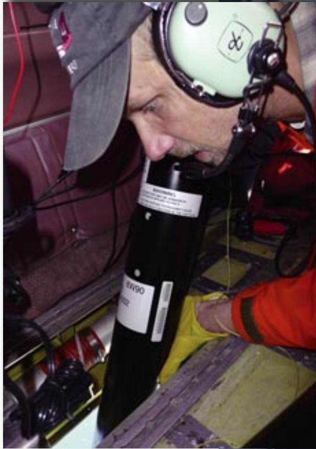
ABOVE: Sonobuoy about to be deployed from the belly port.
