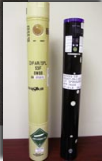
ABOVE: Parts of a USSI-Q53F sonobuoy after being removed from its housing.
