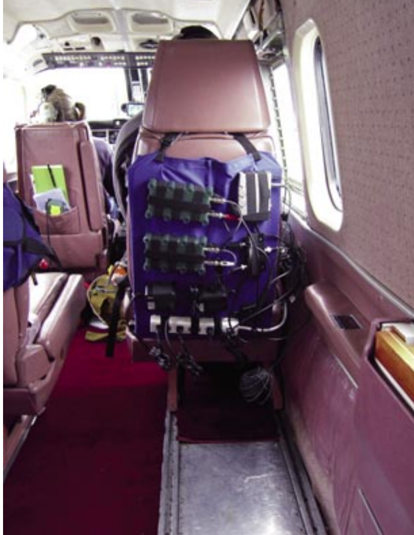
Small spaces require efficient set-up—acoustic receiving and processing equipment on rear of plane seat; “belly port” through which sonobuoys will be deployed is seen below.
