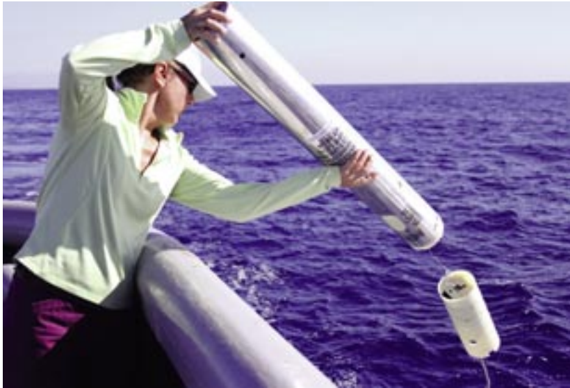
An example of manually deploying a sonobuoy from a ship. Julie Rivers, Natural and Marine Resources Program manager at Commander, U.S. Pacific Fleet deploying a sonobuoy to listen for marine mammals in Hawaii.
