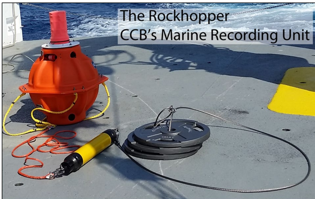
Figure 2: The Rockhopper marine recording unit developed by the K. Lisa Yang Center for Conservation Bioacoustics at Cornell University, Ithaca, New York, U.S.
