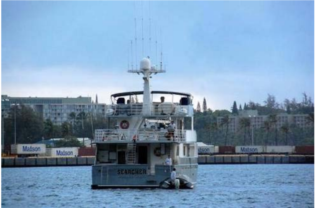
Figure 3. Stern view of the M/V Searcher showing three decks, including the top covered observation deck or flying bridge.
