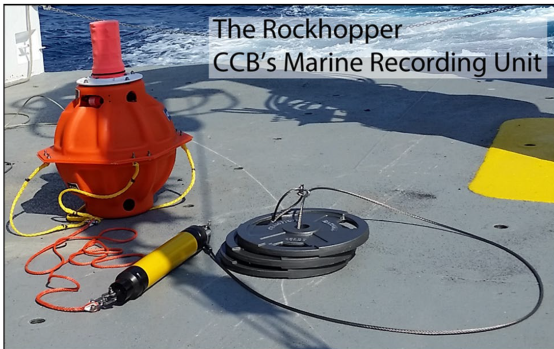
Figure 2: The Rockhopper marine recording unit developed by the K. Lisa Yang Center for Conservation Bioacoustics at the Cornell Lab of Ornithology, Cornell University, Ithaca, New York, U.S.
