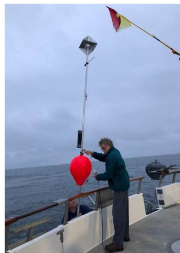
Deploying DASBR from a dive platform
