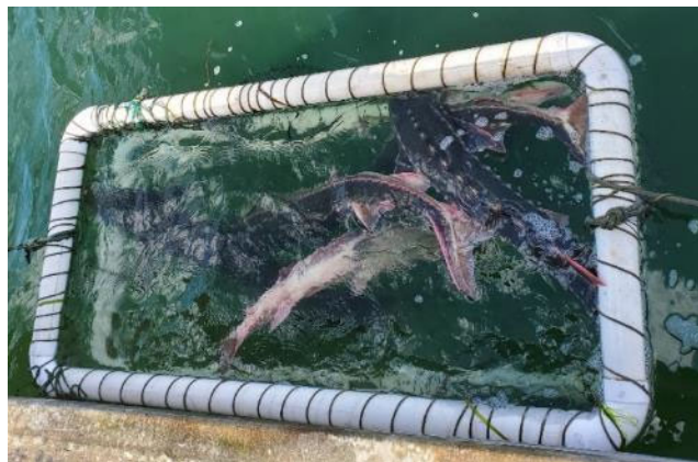
Figure 1. Image of the fish car attached to the side of the research vessel. This equipment is used to provide access to fresh oxygenated water for captured sturgeon prior to sampling and release for the purpose of decreasing handling stress and increasing the likelihood of post-release survival.
