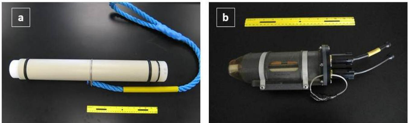
**Figure 3.2.** Photographs of the passive acoustic monitoring devices used to monitor the occurrence and distribution of bottlenose dolphins in the New River, North Carolina. (a) C-POD – an echolocation click train detector and (b) DMON – a digital, archival acoustic recorder.
