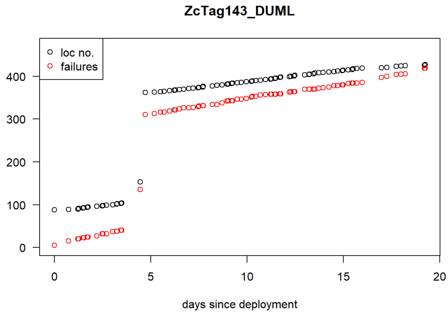
Figure 25. FastGPS successful fixes (black circles) and failures (red circles) over deployment duration in which FastGPS data collection was active for ZcTag143_DUML.
