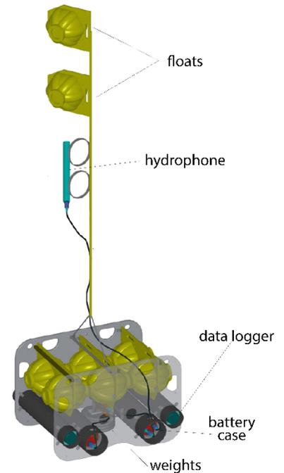
**Figure 3.** Schematic of a HARP seafloor package
