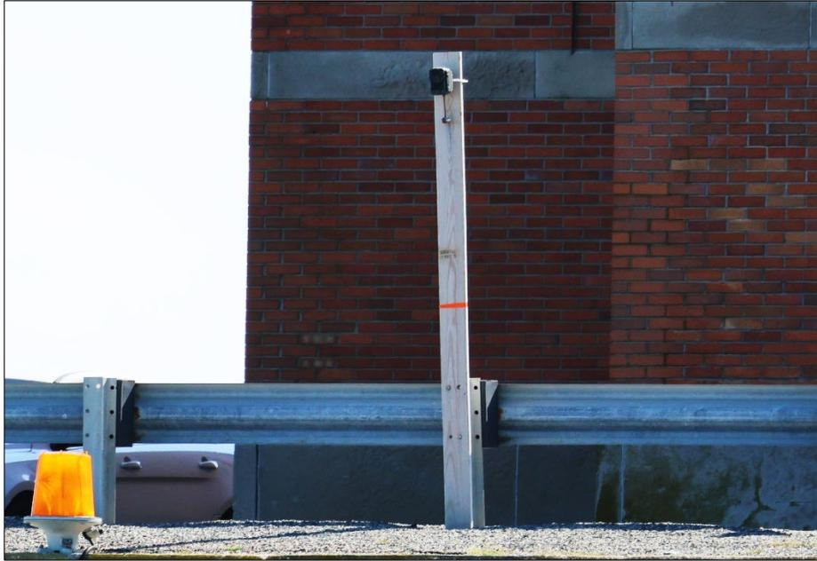
*Figure 2-6. Image of camera installed on elevated 2x4 wooden post for the 2020/2021 and 2021/2022 seasons. Photo by D. Jones, Naval Facilities Engineering Systems Command Atlantic*
