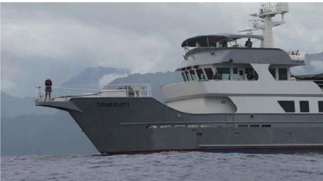
Figure 2. The r/v Searcher. Visible in this photo is the covered flying bridge from which the bird, monk seal, and cetacean/sea turtle survey takes place and the bow sprit which is the best position for cetacean photography.
