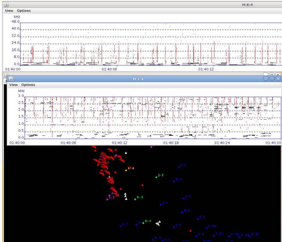
Figure 3- The upper and middle show binary spectrogram plots of Sperm whale echolocation clicks. The lower image indicates the whale localization in red with the hydrophones in blue.
