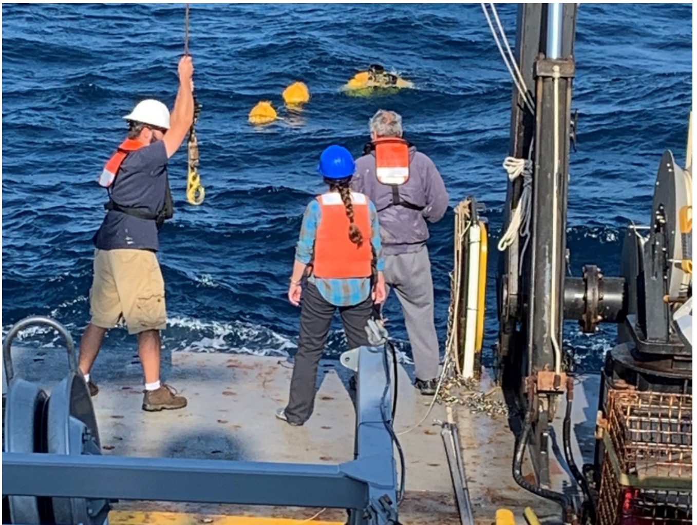
Figure 5.2. Image of a HARP recovery. The HARP (high-frequency acoustic recording package) is released from the seafloor using an acoustic signal transmitted by a shipboard transducer and must be spotted visually once it surfaces. The ship then approaches and a hook is thrown to pull it in. The HARP is then attached to the ship's crane and lifted onto the deck.
