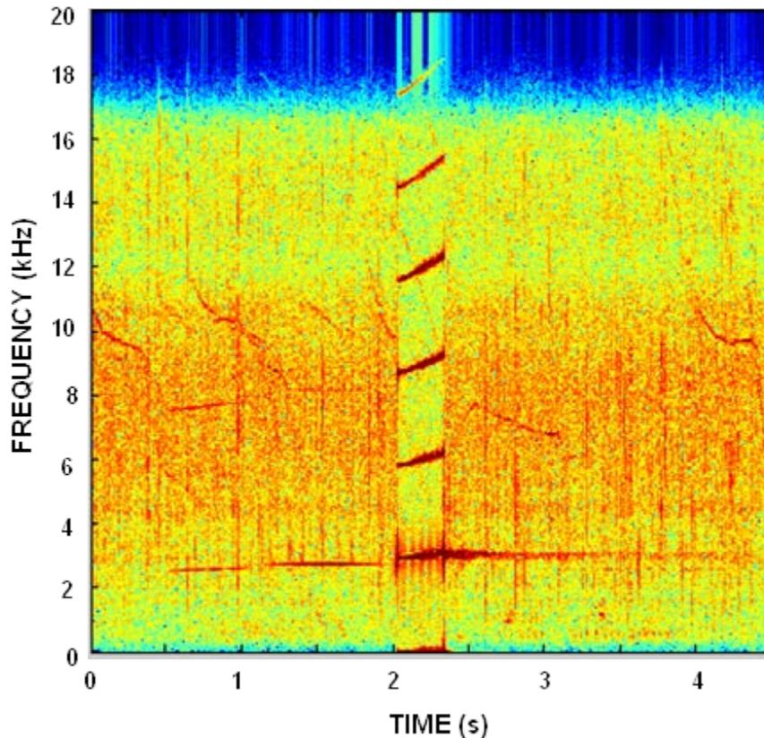
**Figure 6. A sonar signal that saturated the EAR, producing many harmonics. Dolphin whistles can also be seen in the spectrogram. The peak-to-peak sound pressure level that causes EAR saturation is approximately 160 dB re 1  $\mu$ Pa.**
