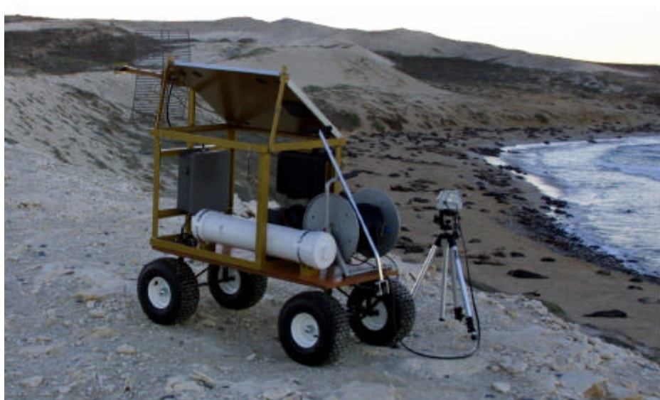
FIGURE 3.2. View of a wagoncam, which unlike other portable video cameras, can transmit its signal back to a centralized location where it is recorded. (Photograph by U.S. Navy)
