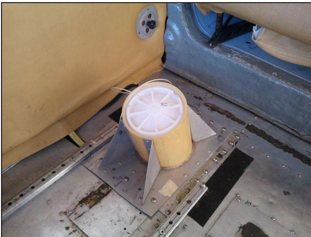
*Photo 1. View of sonobuoy chute from inside the Partenavia aircraft. The white disk is a cover that keeps the wind from blowing inside the aircraft, and is removed immediately prior to sonobuoy launch.*
