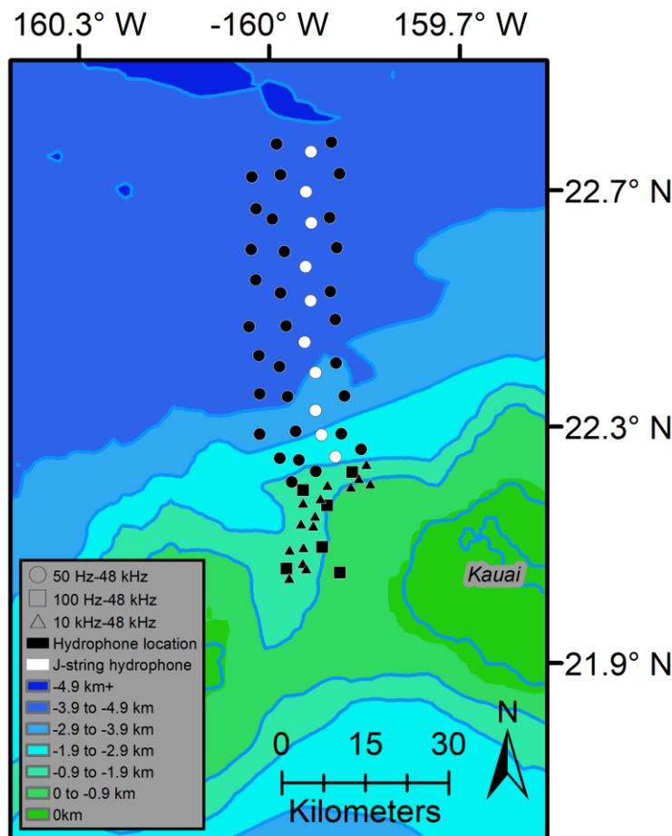
**Figure 1: Map showing approximate locations of the 62 hydrophones that have been recorded since August 2012. The 47 broadband hydrophones are depicted as circles (frequency response 50 Hz-48kHz) and squares (frequency response 100 Hz-48kHz). The high-pass hydrophones are depicted as triangles (10 kHz-48kHz). The white circles indicate the J-string hydrophones that went out in June 2017.**
