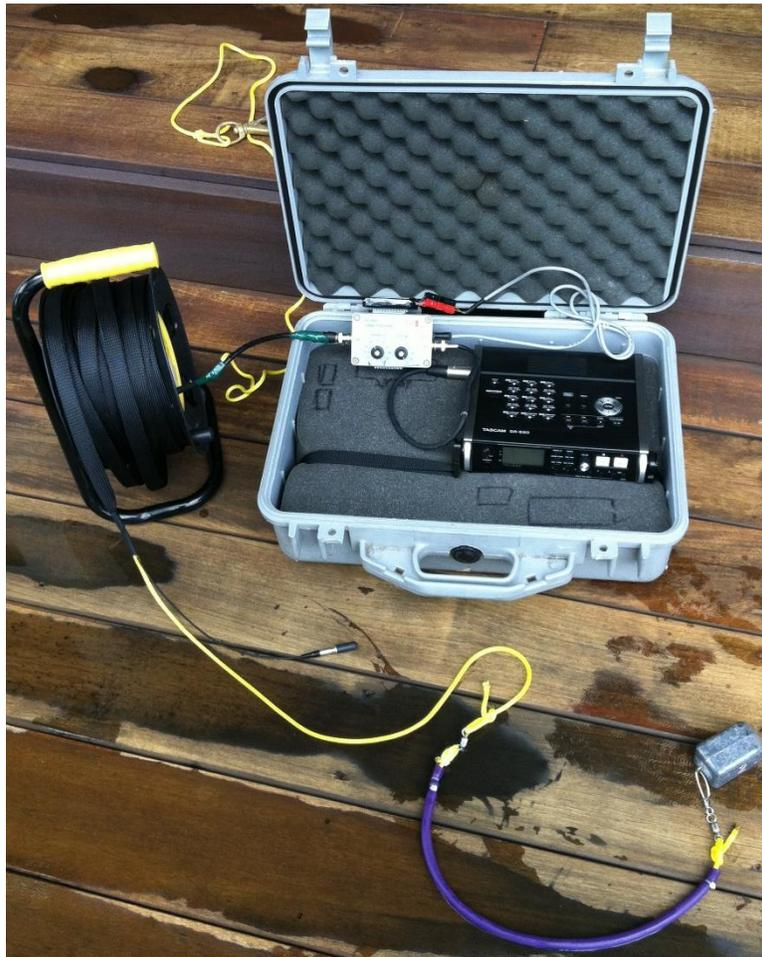
**Figure 2: Recording setup deployed for in situ near surface measurements in February and August 2014. Note the one-pound weight and lack of depth recorder. The analog-to-digital recorder was also different from later recordings.**
