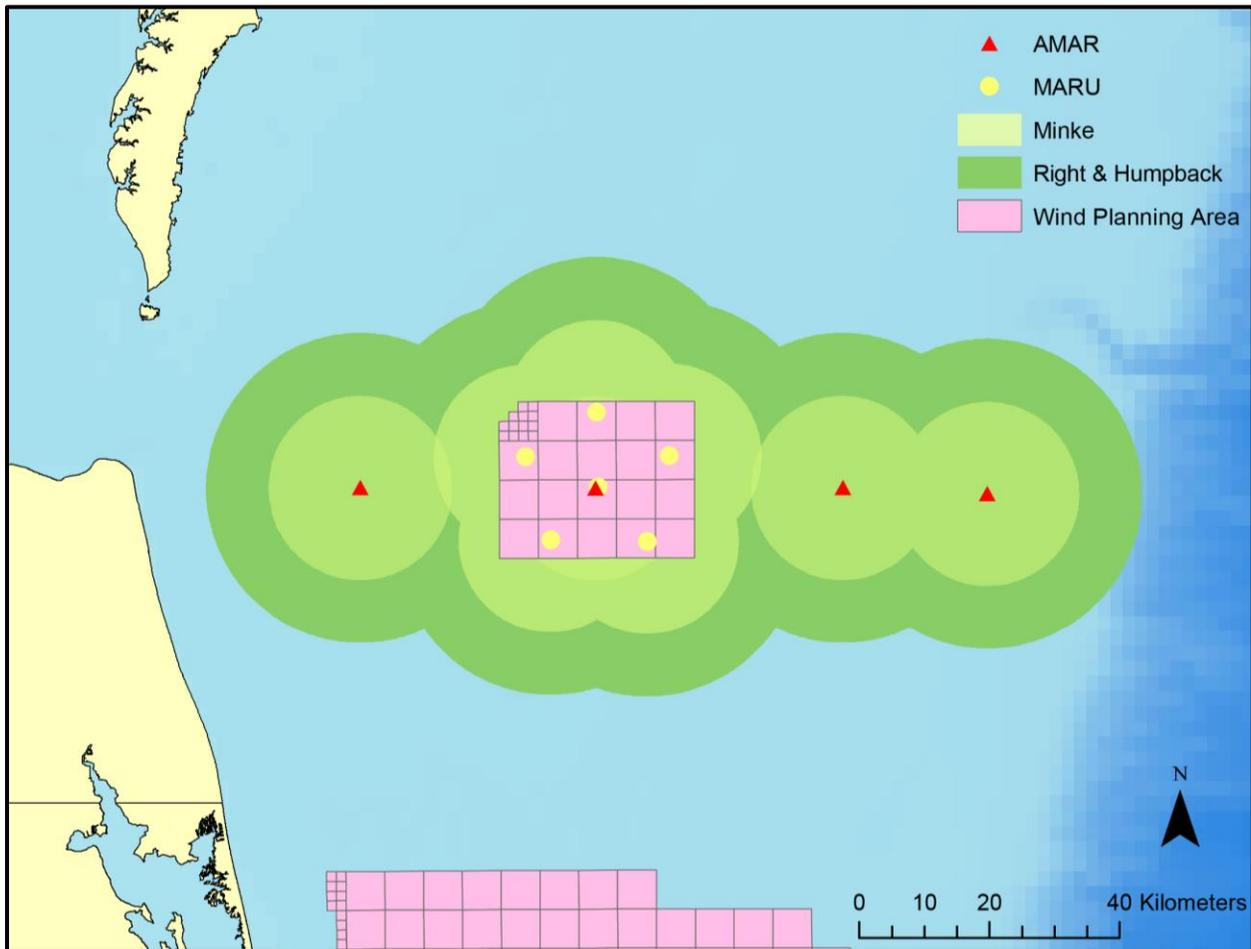
**Figure 64. Map of low-frequency (MARU) and high-frequency (AMAR) passive acoustic recorders deployed across the continental shelf off the mouth of Chesapeake Bay. Green shading indicates estimated detection ranges for minke, North Atlantic right, and humpback whales.**
