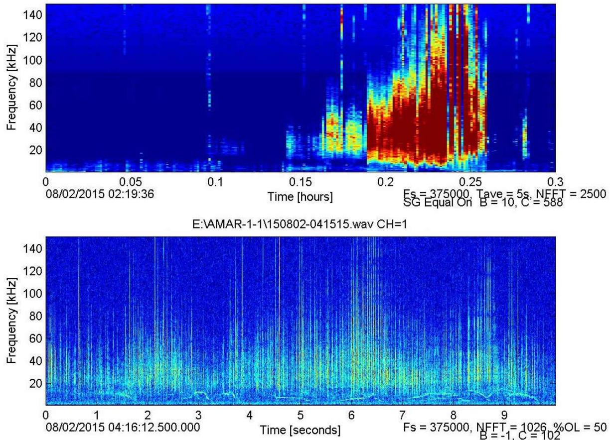
**Figure 67. Long-term spectral average plot (top) indicating an odontocete encounter recorded with the inshore high-frequency recorder in August 2015. The spectrogram (bottom) shows the corresponding whistles (tonal sounds in the 10–20 kHz range) and echolocation clicks (broadband transient signals).**
