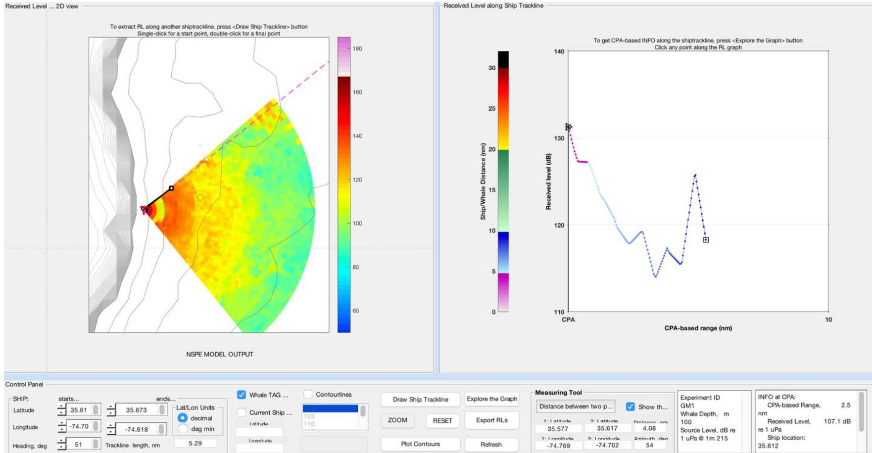
**Figure 56. Modeled received levels for Zc17\_234a (at location indicated by T) at 100 m depth from *in situ* acoustic propagation assuming the (F/V) Kahuna at starting source location selected for CEE#2017-01 (35.548; -74.770).**
