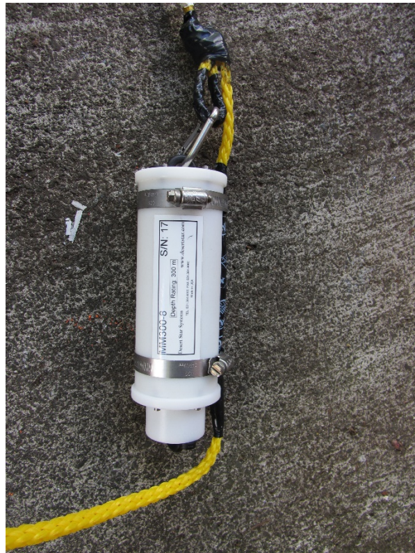
Figure 2. MicroMARS recorder included in the surface array.
