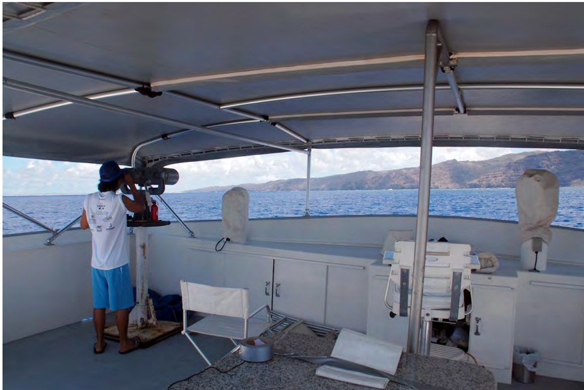
Figure 5. Flying bridge and port big-eye binocular. The starboard big eye is to beyond the camera view to the right.
