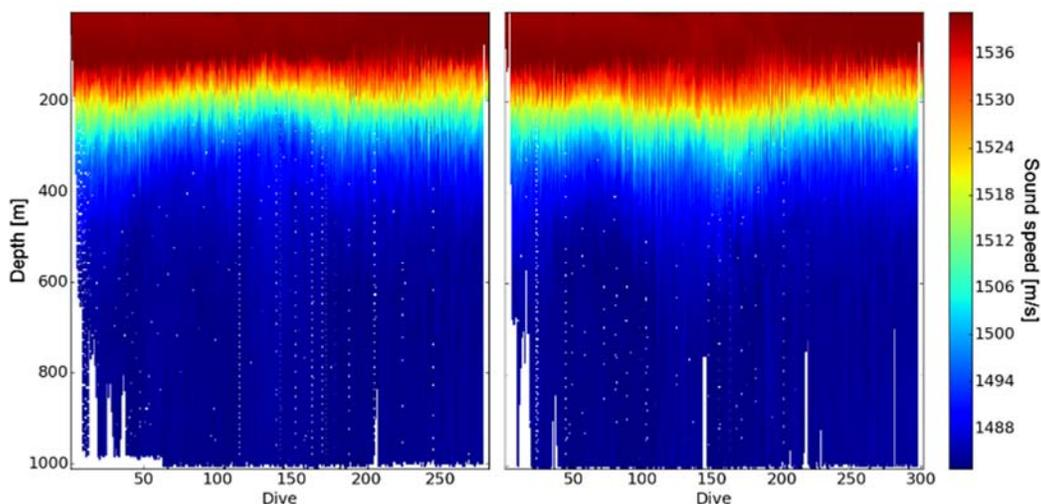
Figure 7: Sound-speed profiles recorded with SG178 (left) and SG204 (right).
