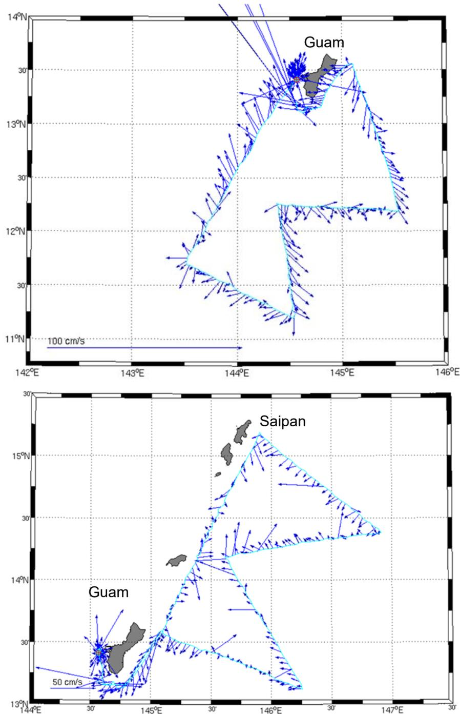
Figure 8: Depth-averaged currents measured with SG178 (top) and SG204 (bottom).
