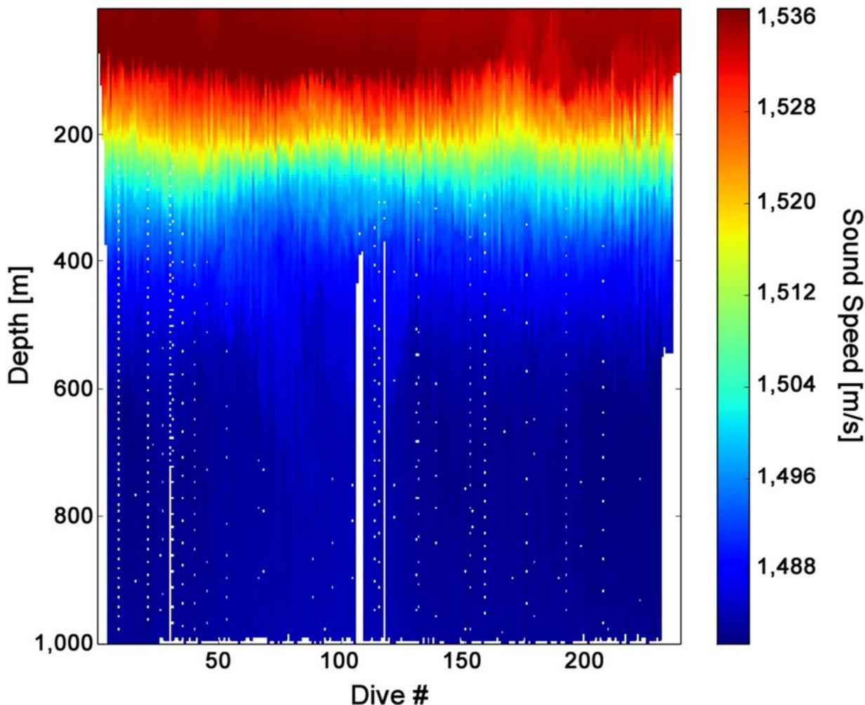
Figure 7: Sound-speed profiles recorded with SG203.
