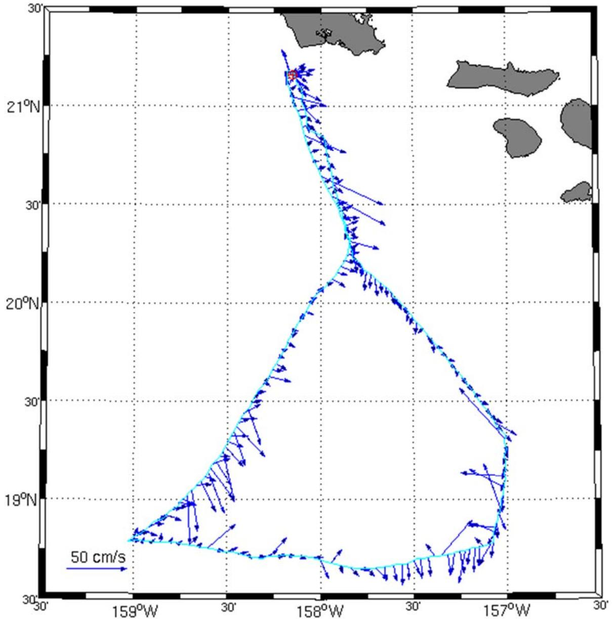
Figure 8: Depth-averaged currents measured with SG203.
