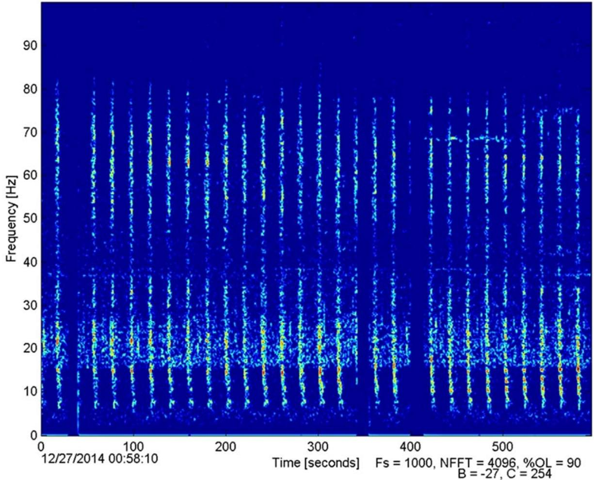
Figure 37: Seismic airgun signals recorded with SG203 on 27 December 2014.
