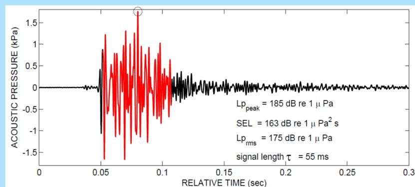
Typical time series of underwater sound pressure from impact pile driving and corresponding metrics (peak pressure, RMS, and SEL) computed automatically by the USLM. The region in red constitutes 90% of the energy from which the RMS and SEL metrics are derived.
